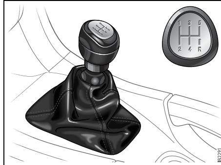
Gear positions, 5-speed
